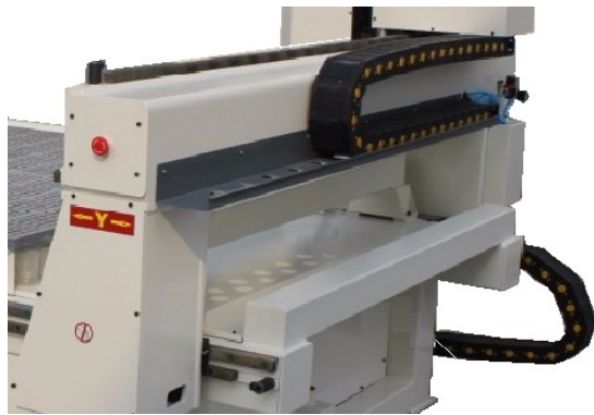
X 25 mm Y Axis 25 mm Linear Rail, Rack-Pinion
